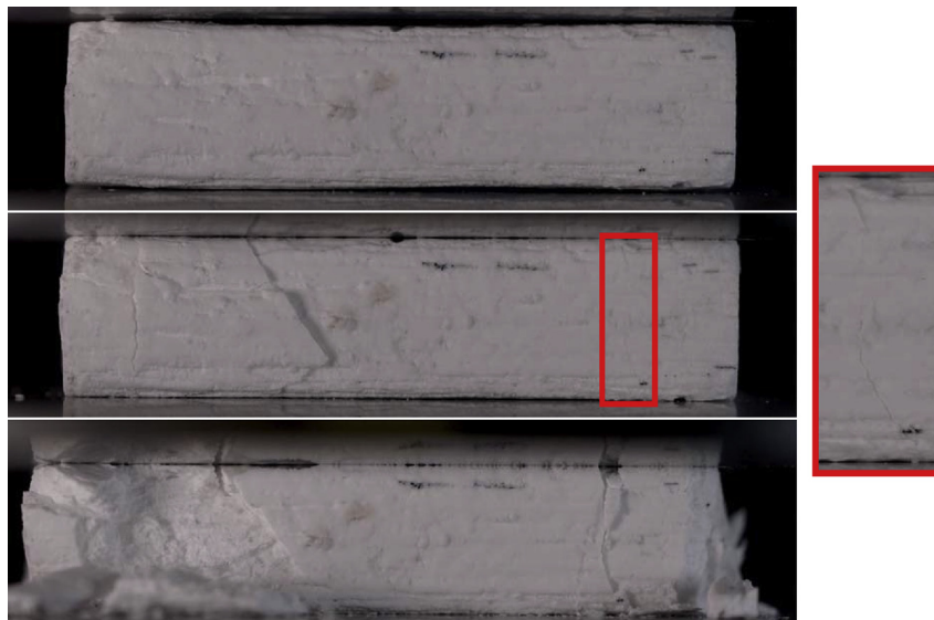
Fig. 10. A sequence of photos showing progressive failure during uniaxial compression orthogonal to the grain of a BA prismatic sample (from set #4, geometrical and mechanical properties reported in Table 4). BA, biomorphic apatite.
